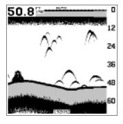
"AUTO" at the screen's top center shows that the sonar is in the automatic mode, freeing you from sensitivity, range, and noise rejection adjustments. The "192 KHZ" at the bottom of the screen shows that this chart is operating at 192 kHz. You can switch the full chart between 192 and 50 kHz.
